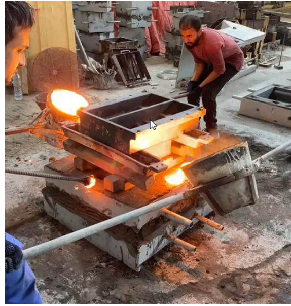
POURING OF MELTED ALUMINUM
